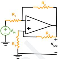
b) Now,  $R_1 = R_3 = 2 \text{ k}\Omega$ , and  $R_4 = 3 \text{ k}\Omega$ . Design the amplifier by choosing the value of  $R_2$  so that the gain is positive 50.
